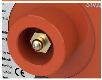
The WH-HSB snatch block incorporates a grease nipple, allowing additional lubrication to be injected into the snatch block. This enhances operational efficiency by ensuring low friction smooth operation, and reduces unnecessary maintenance.
