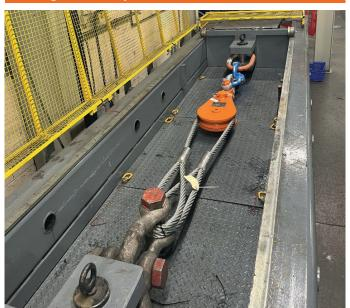
The WH-HSB snatch block is subject to rigorous testing and quality assurance processes. Moreover, our testing has been independently witnessed and verified by Apave TIV UK Limited. This third-party verification included proof load testing in accordance with EN13157:2004+A1:2009, dimensional verification before and after proof load testing, and minimum break load testing (i.e., testing to four times the working load limit) under a static load for 10 minutes.
